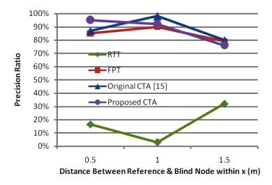
Fig. 11. Precision when acceptable estimation error is within 1.0 m at different distances (x meters) (Precision: four reference nodes).
