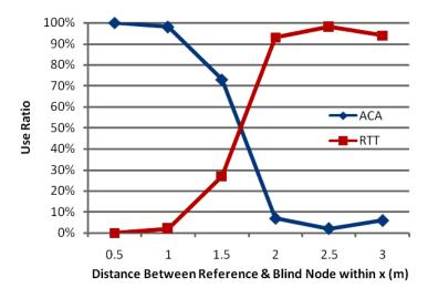
Fig. 13. Usage ratio of the ACA and RTT modes.
