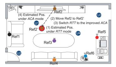
Fig. 6. Process of switching the RTT mode to the improved ACA mode by moving a reference node.
