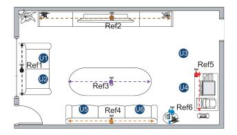
Fig. 19. Experimental environment of the movable reference nodes.
