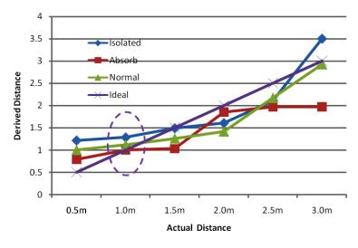
Fig. 9. Results of transferring the RSSIs to distances using formula (9), where (A, n) = Isolated (6, 4); Absorb (45, 10); Normal (30, 9).
