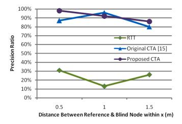
Fig. 15. Precision when error distance is within 1.5 m (precision: eight reference nodes).
