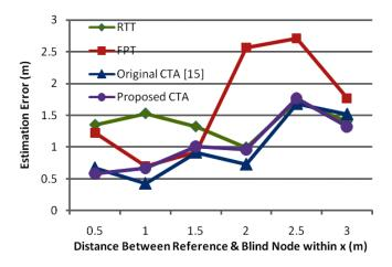
Fig. 10. Estimation error vs. the distance between the reference nodes and the blind node at distance  $x(m) = \{0.5, 1.0, 1.5, 2.0, 2.5, 3.0\}$  m (accuracy: four reference nodes).
