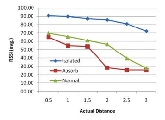
Fig. 8. Average RSSIs in different environments: Isolated, Absorb, and Normal. For example, thresholds can be defined as [mean  $-1.0^*\sigma$ , mean  $+1.0^*\sigma$ ], where  $\sigma$  is the standard deviation.
