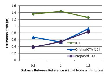
Fig. 14. Estimation error vs. distance between the reference nodes and the blind node at distance  $x(m) = \{0.5, 1.0, 1.5\}$  m (accuracy: eight reference nodes).
